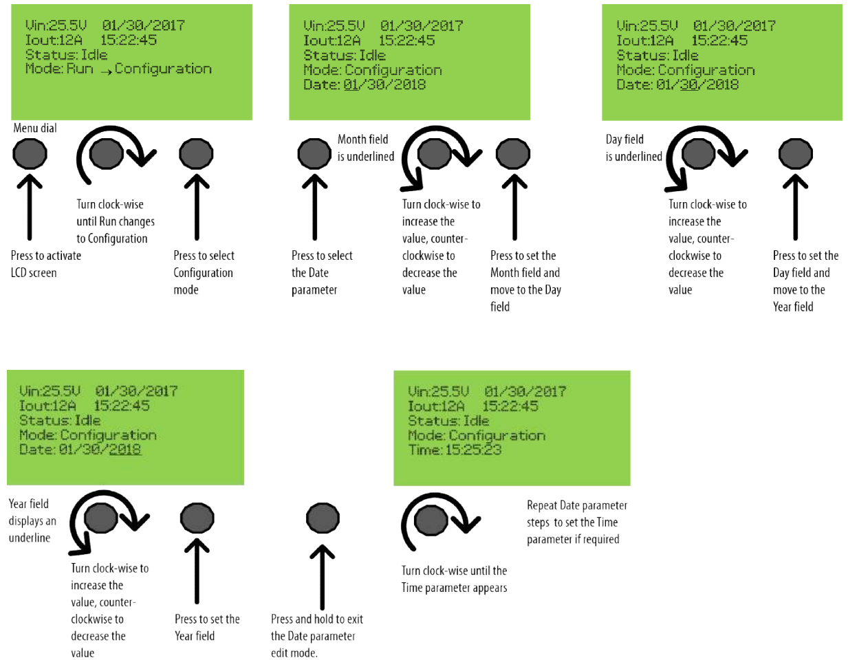
Figure 15: Setting parameters via LCD and Menu dial
